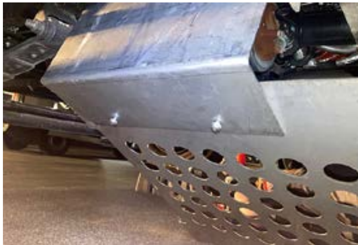
Forward tamper-proof screws
